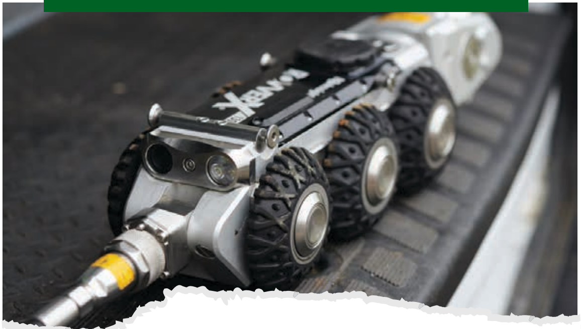
Pipe Inspection: Battery Operated Pipe Crawler Inspection System on FSA23-EQU21.1
