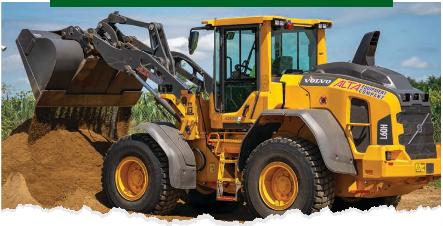
Loader: Wheel Loader - 3.0 cubic yd. on FSA23-EQU21.1
