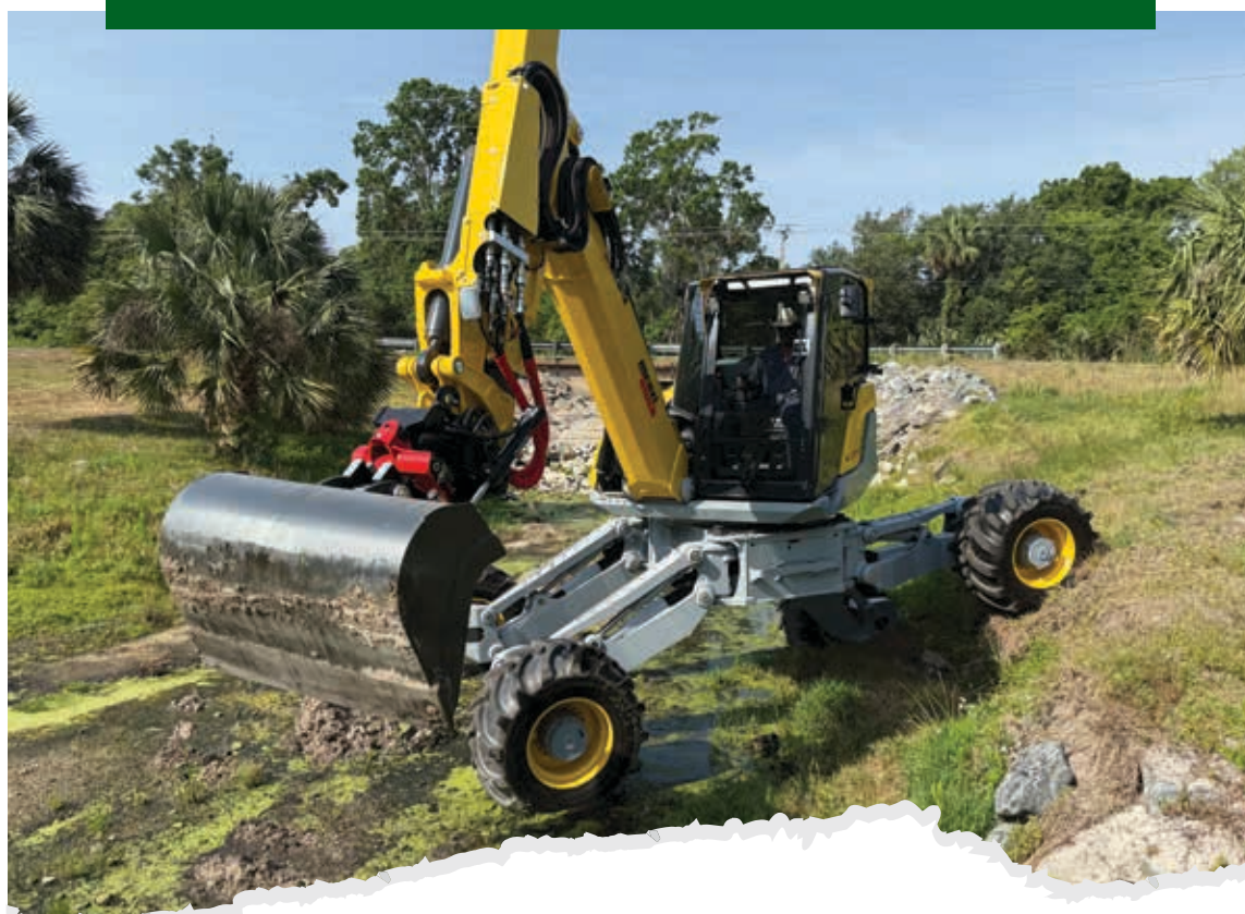
Excavator: All Terrain Walking Excavator on FSA23-EQU21.1
