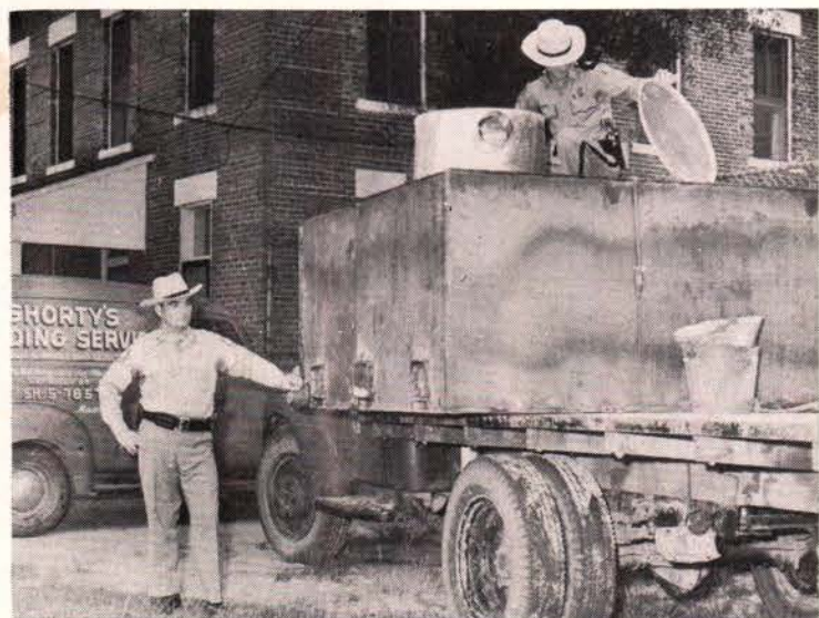
MACCLENNY—MOBILE MOONSHINE STILL —Baker County Deputy Sheriff G. W. Rhoden (left) and Florida Highway Patrol Trooper L. B. Boyette inspect a mobile moonshine still they confiscated recently. The "cooker" fired with butane gas, was built on a flatbed truck and additional equipment was carried in a panel truck. Once the cooker was loaded with a batch of fermented mash it could go into business anywhere as long as a source of water was available to cool the condenser. (Photo courtesy Florida Times-Union.)
