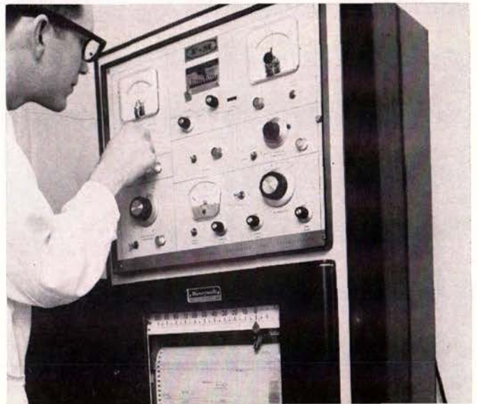
The Gas Chromatograph is the latest addition to the Sheriffs Bureau Crime Laboratory's arsenal of scientific instruments. It can be used to analyze many different substances gathered as evidence in criminal investigations, including petroleum products, narcotics, blood and alcohol. In arson investigations it helps officers to determine whether gasoline, kerosene or other inflammable materials were used.
