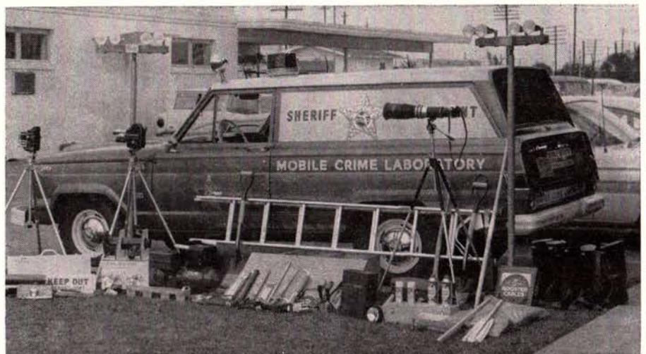
WEST PALM BEACH — NEW MOBILE CRIME LAB — Equipped for on-the-spot analyses is Sheriff Martin Kellenberger's mobile crime laboratory under direction of Capt. Thomas Nunn, chief of the Bureau of Technical Services. The vehicle has a portable gasoline-operated generator, two stands with five 150-watt bulbs mounted on each, cameras, fingerprint equipment, rope to seal off a crime area, a two-man inflatable raft, magnet to search for weapons underwater, a ladder, megaphone, first aid kit, and other items to suit the scene of the crime. The equipment is used by detectives and two experts in Nunn's department, William H. (Pete) Ragsdale, a forensic chemist, and Ben Green, fingerprint identification officer. (Photo courtesy of West Palm Beach Post.)
